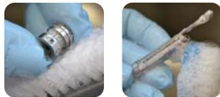
**3. STAGE: WASHING** The parts should be brushed with a soft bristle brush, paying particular attention to joints, serrations and racks. The joints should remain open, being brushed on both sides, the serrations brushed in both directions towards the serra itself and the racks brushed in both directions towards the teeth.
