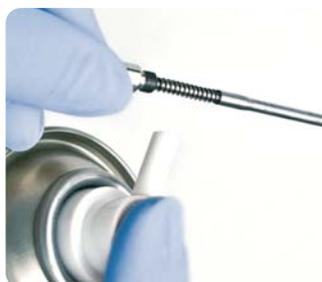
**5. STAGE: LUBRICATION** (for detachable parts). After rinsing, it must be ensured that the instrument is free of any dirt or other residues. Every instrument must be lubricated, using water-soluble and non-corrosive lubricant, suitable for medical application, with special attention to the joints of the articulated instrument.
