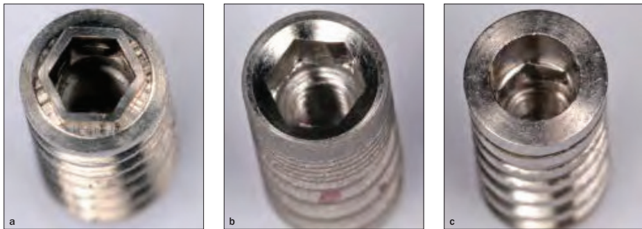
Fig 1 Implant connection configurations tested. (a) EH, (b) IH, (c) MT.
